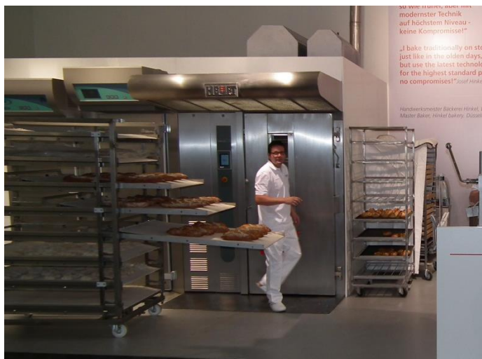
Image of similar “Combination Trolley” with setters pulled out to remove baked products.
